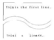
2. The self test continues until the paper runs out or until you press the **ON LINE** button. To stop the test, press the **ON LINE** button.
